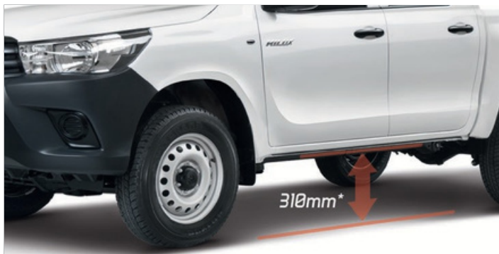
GROUND CLEARANCE - Keep Operations Going and Deliver No Matter What the Road Condition. 195mm (Hilux 4x2J) and 310mm (Hilux 4x4J)
